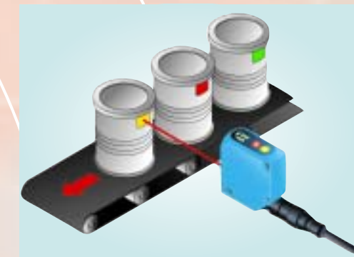
Detection of different-coloured labels
